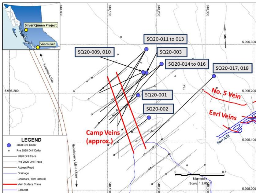
Figure 1: Plan Map of Phase I+II Drilling on the Camp and No. 5 Veins
